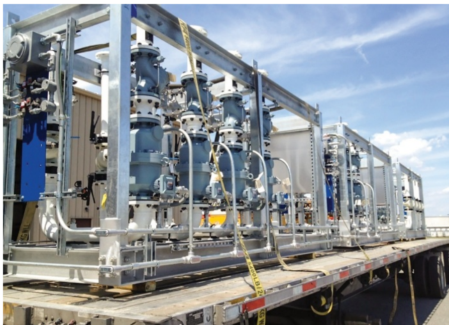
FIG. 2. Small modular process skid.
