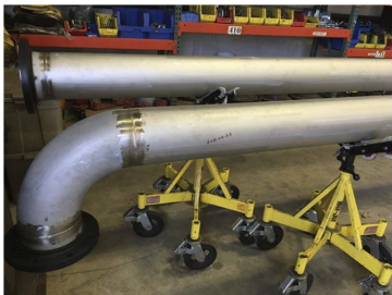
Figure 5. Large diameter stainless steel pipe fabrication.
